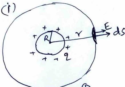
Let  $\sigma = \frac{q}{4\pi R^2}$  be the surface charge density of spherical shell.
