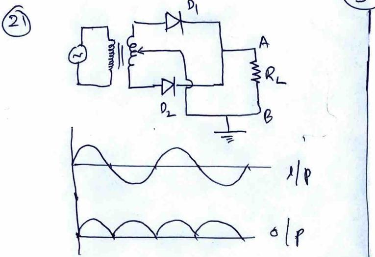
During +ve half cycle,  $D_1$  is forward biased and  $D_2$  is reverse biased.  $D_1$  will conduct and a current flows from A to B.
